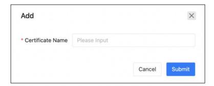
Each certificate entry created here is for an OpenVPN client. Download the certificate and extract files inside the package, 3 files you'll get and they should be uploaded on a client to be able to connect to this server.
