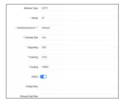
In the **Signaling** dropdown list you should select SS7, **Framing** and **Coding** should use default value. Below in the **SS7 Settings** section set the detailed SS7 parameters.
