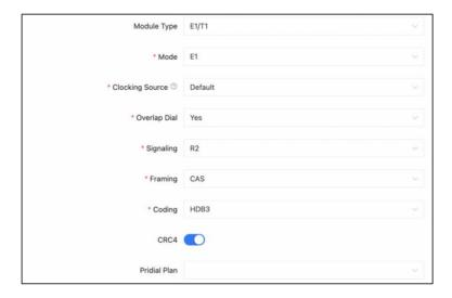
In **Signaling** field select R2, **Framing** and **Coding** should use default value. Below in the R2 Signaling Settings section set the R2 parameters.
