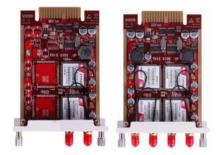
2GSM/4GSM module provides 2/4 GSM channels, it can be installed on T200/T600 for making and receiving phone calls from GSM network. It is designed with SIM900 for the global market, SIM900 is a quad-band GSM engine that works on frequencies GSM 850MHz, EGSM 900MHz, DCS 1800MHz and PCS 1900MHz.
