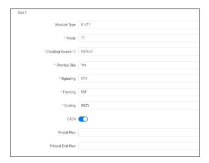
T1 runs on same signaling types as E1 mode. And T1 uses different Framing and Coding methods, configure these parameters according to the details provided by the telephony provider. In most cases CRC4 is not needed for T1 circuit, enable it only when the provider requires it.
