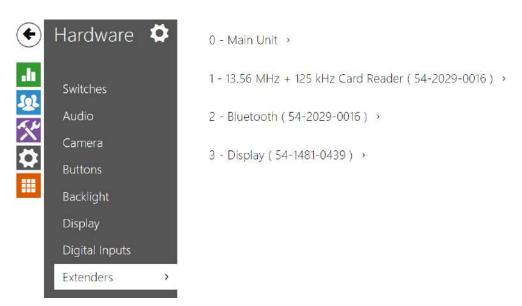
The **2N P Verso** and **2N P Style** intercoms can be extended by means of extending modules connected to the intercom basic unit via a VBUS. The following modules are available:
