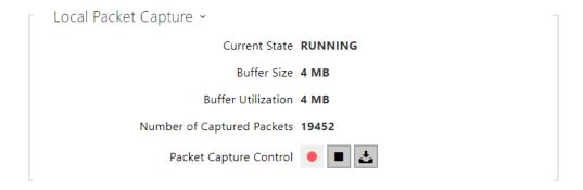
When the local capture buffer is full, the oldest packets are rewritten automatically. We recommend that you lower the video stream transmission rate below 512 kbps while capturing packets locally. Press to start, to stop and to download the packet capture file.
