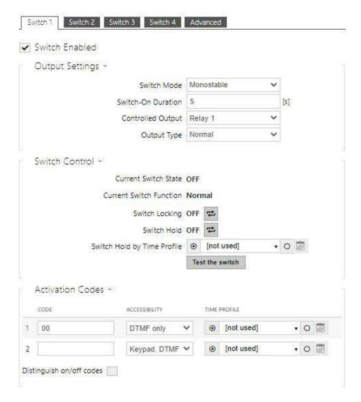
Enable the switch in the Switch Enabled parameter in the **Hardware / Switches / Switch 1** tab, set the Controlled Output to the intercom output to which the electric door lock is connected. Now set one or more activation codes for the electric door lock switching.
