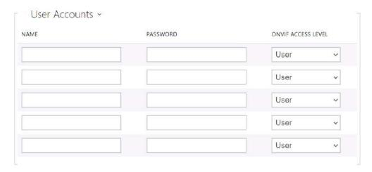
Be sure to set one user account at least and the proper access level (according to ONVIF specification and used VMS) to achieve full ONVIF functionality. Without this, the basic functionality is only available.
