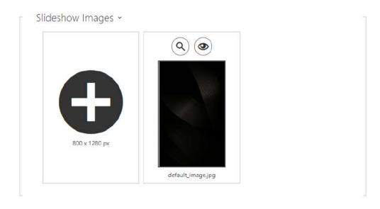
The recommended resolution is 800 x 1280 px for images and 400 x 640 px for video files in  $2N^{\circ}$  **IP Style**. The device automatically adjusts images with a different resolution value.
