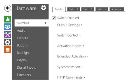
Switches provide a very flexible and efficient control of such intercom peripherals as electric door locks, lighting, additional ringing signalling, and so on. **2N IP intercoms** allows you to configure up to 4 (depending on model types) independent all-purpose switches.
