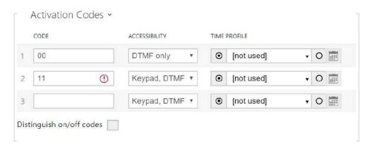
The table above includes a list of universal codes that help you activate switches from the phone or intercom keypad. Up to 10 universal codes can be defined for each switch (depending on the particular intercom model).
