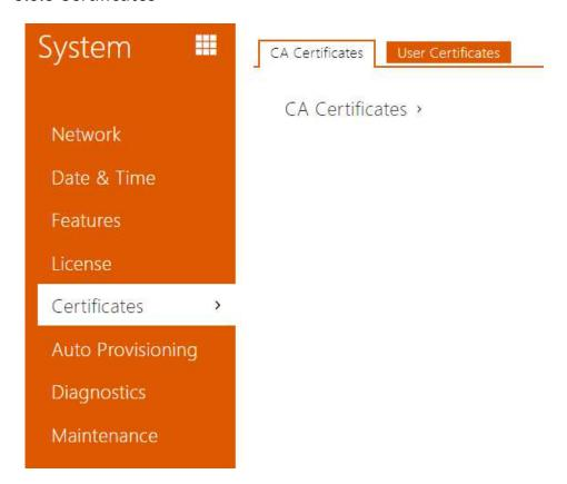
Some **2N IP intercom** network services use the Transaction Layer Security (TLS) protocol for communication with other LAN devices to prevent third parties from monitoring and/or modifying the communication contents. Unilateral or bilateral authentication based on certificates and private keys is needed for establishing connections via TLS.
