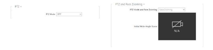
• PTZ Mode – enable the PTZ (Pan-Tilt-Zoom) function to control the camera display area during the call via DTMF (GOLD license required) from your IP phone numeric keypad. If the PTZ mode is enabled, you can control the camera via your IP phone numerical keypad. Press the \* key to enable/disable PTZ. The meanings of the IP phone keys in the PTZ mode are as follows:
