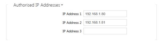
• IP Address 1-4 – set up to 4 authorised IP addresses from which you can log in to the RTSP server. If none of the four fields is completed, any IP address can be used for login.
