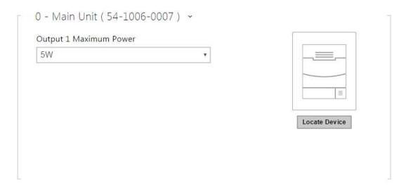
• **Locate Device** – optical and acoustic signaling of a device. Note: Optical signaling is possible only if the device is equipped with control backlight (Verso, Base, Vario, Force, Safety and Uni). If a speaker is not integrated in the device, make sure than an external speaker is connected (Audio Kit and Video Kit) to use sound signaling.
