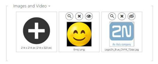
Make sure that the image / video resolution is 214 x 214 or 214 x 320 pixels up to 2 MB. Other sizes will be adjusted to the display resolution automatically.
