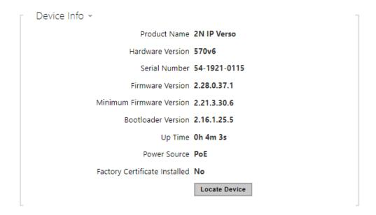
• Factory Certificate Installed – specify the user cerificate and private key to be used for verifying the intercom authorization to communicate with the third party device server.
