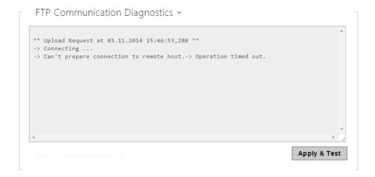
Click **Apply & Test** to save the current FTP server configuration, load the camera image and save the image to the FTP server. The window above displays the FTP server communication details during saving.
