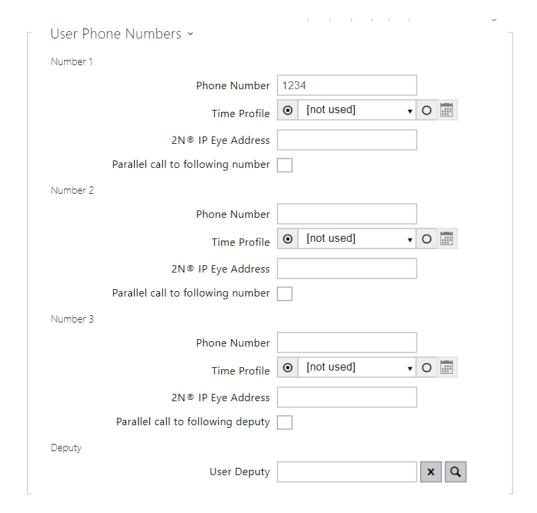
You can also use the **2N IP intercom** with one or more IP phones without a SIP server. Use the Direct SIP Call. For outgoing calls and enter the called phone SIP address (sip:phone\_number@phone\_ip\_address) instead of the phone number.
