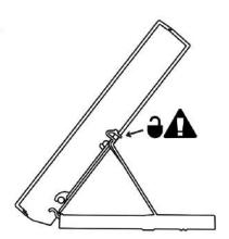
1. Draw the pre-prepared LAN connector through the stand bottom and connect it into the LAN connector socket. Place the cable into the pre-prepared groove in the center of the stand bottom. Unstick the protective foil from the stand antislip surfaces.
