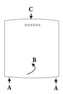
Opening the PABX: »C« is the front of the PABX system. Pull the two plastic springs marked »A« outward until the cover is released. Lift off the cover carefully toward the rear. It can then be easily lifted off. The terminal panel is then visible under the enclosure cover.
