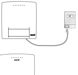
Direct ISDN connection using the ISDN connecting cord supplied with the system at the network termination (NT). This connection option is possible with point-to-point and point-to-multipoint connections. The switches for the terminators in the PABX system must be closed.
