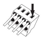
These terminals are for use with ISDN and analog connections. 2 wires can be connected to every connection. Wire diameters can range from 0. 4 to 0. 8 mm. The wire end to be inserted must be stripped of 6 to 7 mm of its insulation. The wires can be removed if pressure is applied with a screwdriver to the terminal bay area designated with an arrow and the wires are removed by pulling lightly.
