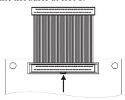
Plug the connection cable into the module so-
