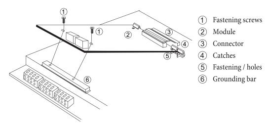
Insert the module into the catches. Note that the restraints must fit into the holes in the module. Using the screws supplied with the package, fasten the module on the grounding bar.
