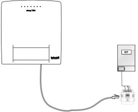
Connection to an ISDN jack installed downstream of the network termination. This connection option is possible with point-to-point and point-to-multipoint connections. Ensure proper connection of the terminating resistors in the PABX, the network termination and the jack.
