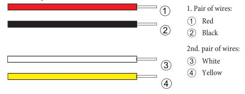
J-YY 2x2x0,6: The four wires are stranded as »star fours«.
